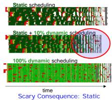
Scary Consequence: Static data decompositions *will not work at scale.*
